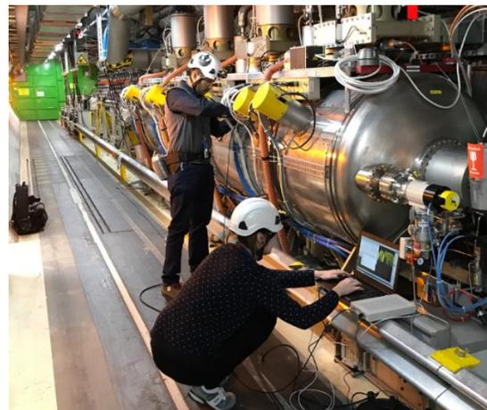
Figure 2. Dr. Castilla and M.S. K Turaj (CERN/BE-RF-SRF) making RF tests in the LHC tunnel. Courtesy of Daniel Valuch, CERN.
