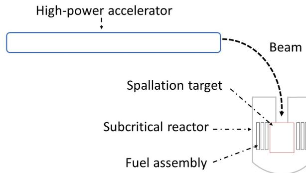
Figure 2. A schematic design of an ADS.
