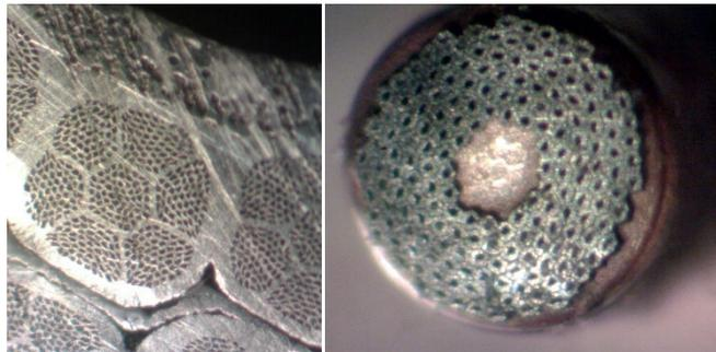
Figure 2. Cable material samples: Bi2212 (left) and NB3SN 8 (right).
