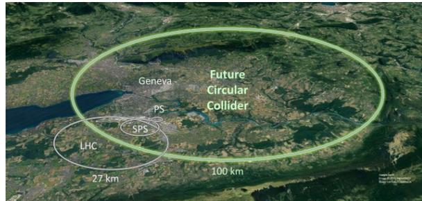
Figure 2. FCC accelerator complex scheme. Courtesy of CERN.
