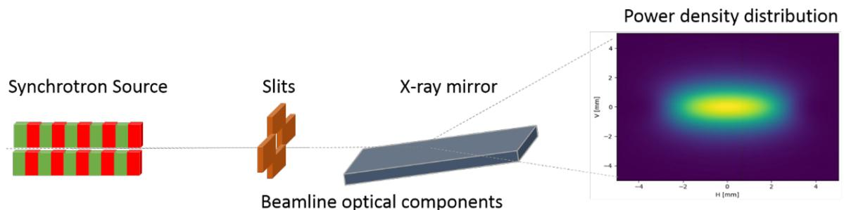
Figure 2. Simulation del studio Example of a basic SR and XRO simulation to study the heat load on a component due the photon beam power.
