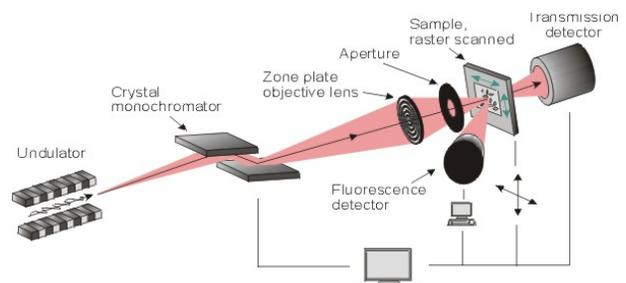
Figure 3. A scanning X-ray Microscope example (ID21, ESRF).
