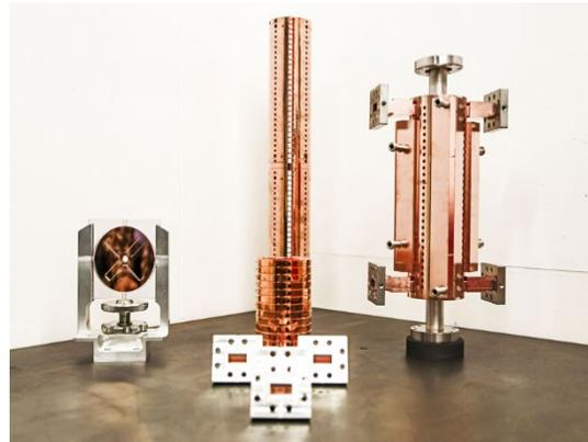
**Figure 2. From left to right and bottom to top: a CLIC disc, waveguides, partial disc stack, full disc stack and full X-Band accelerating structure.**
