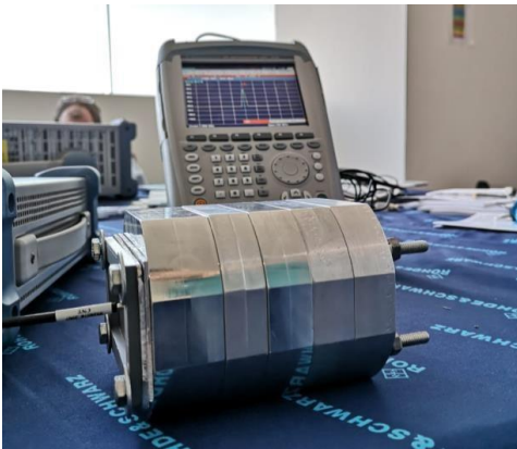
Figure 2 Analysis of the resonance frequencies of an RF cavity using a network analyzer.
